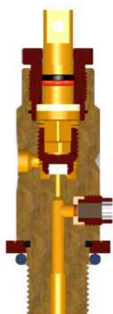
Key [Post] Operated Valve (shown with parallel inlet & PRD)
